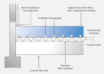
Its high thermal conductivity makes Agilia Screed A perfect for use with underfloor heating.
